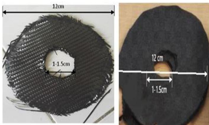
**Figure 2:** carbon fiber cloth and graphite felt
