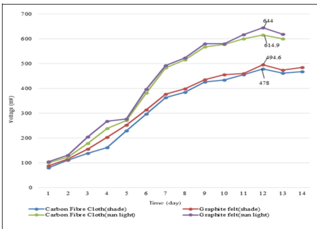
**Figure 7:** variation of average daily voltage with electrode material
