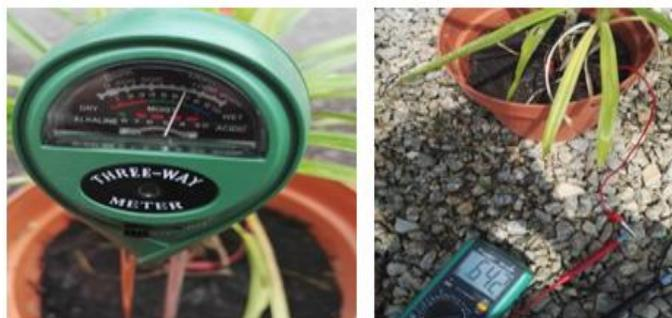
**Figure 4:** Three-Way Meter and Digital multimeter
